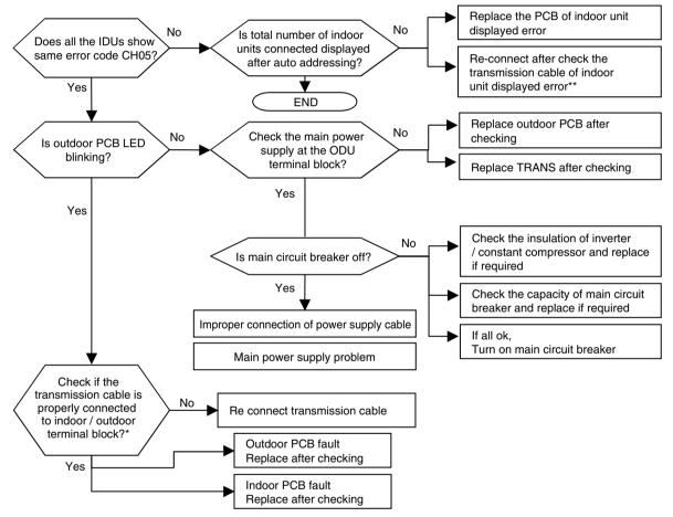
\* (Note1) Transmission from IDU is normal if voltage fluctuation(-9V ~ +9V) exists when checking DC voltage of communication terminal between IDU and ODU
